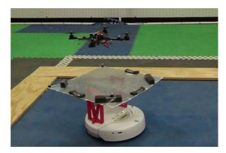
Fig. 1: UAV attempting to land on moving platform.
